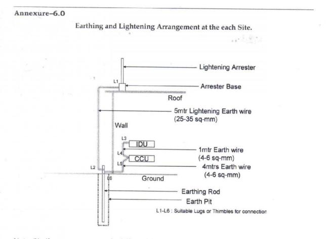
Note: Similar arrangement to be followed for mounting of Lightning arrestor on Pole, except the roof will be replaced by TOP of the pole.
